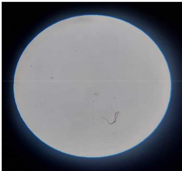
Figure 04: Appearance of microplastic particles under a microscope (Fiber-Shaped Particle).
